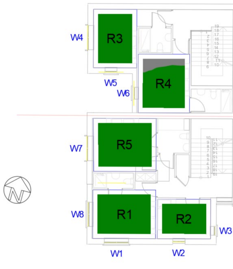
Figure 27: DP-01-02 Second Floor sDA Contours
