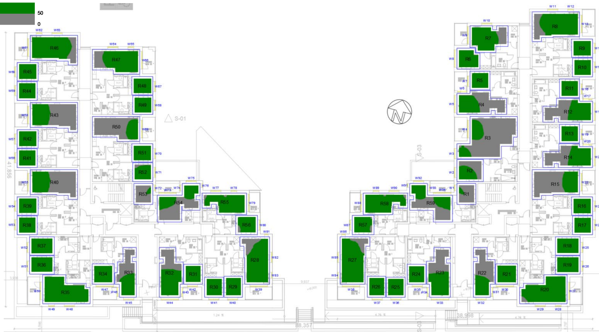
Figure 20: Resi. Apartment Ground Floor sDA Contours
