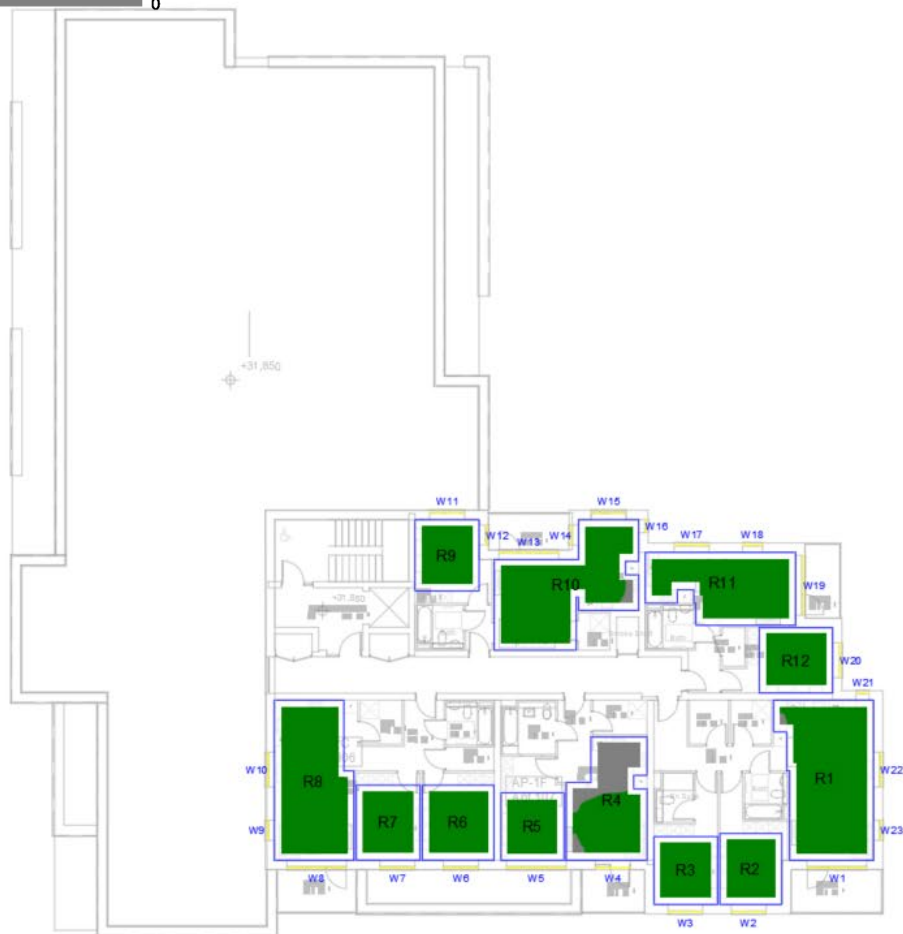
Figure 24: Resi. Apartment Forth Floor sDA Contours
