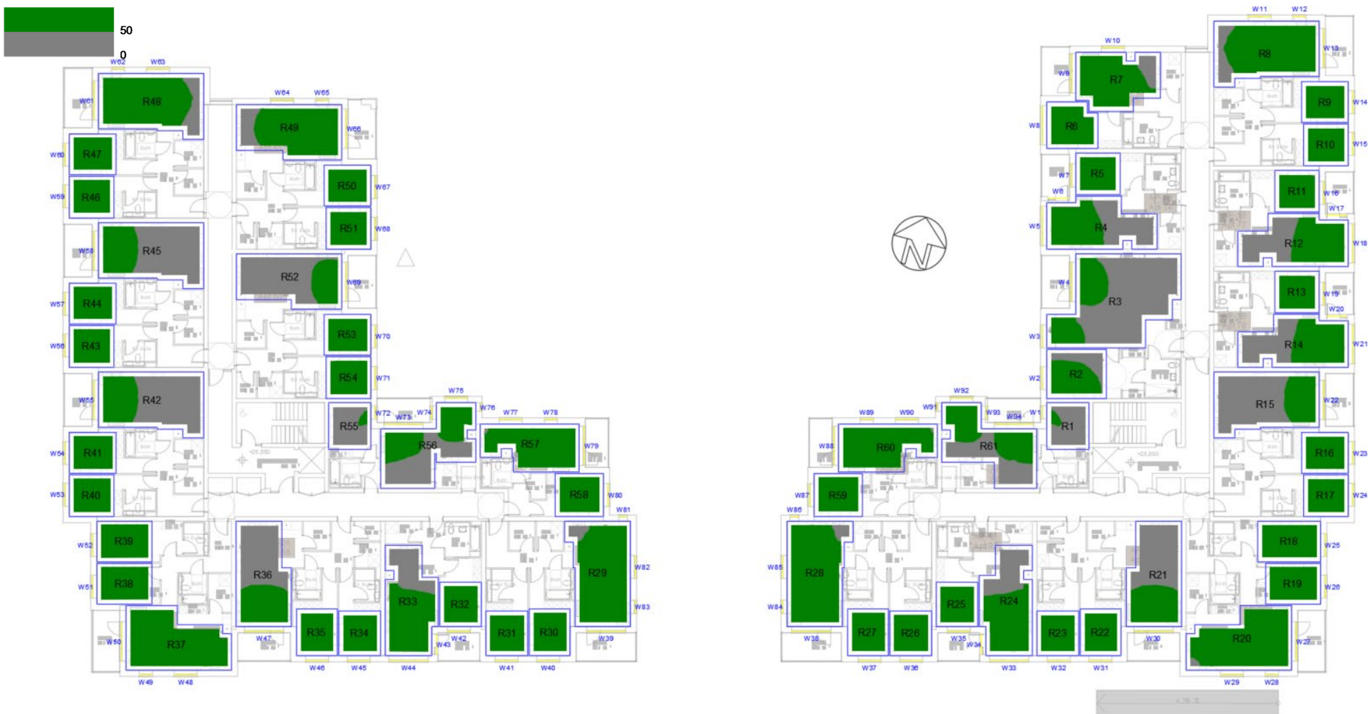
Figure 22: Resi. Apartment Second Floor sDA Contours
