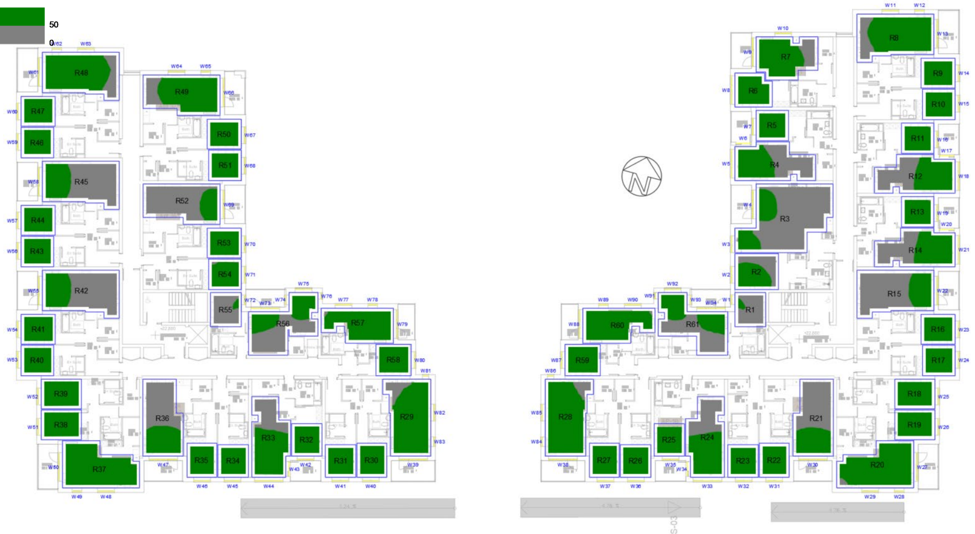
Figure 21: Resi. Apartment First Floor sDA Contours
