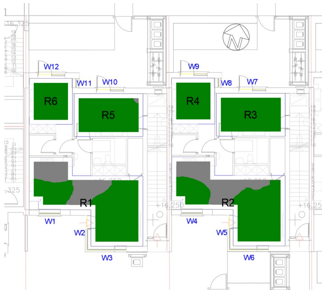
Figure 28: DP-03-04 Ground Floor sDA Contours
