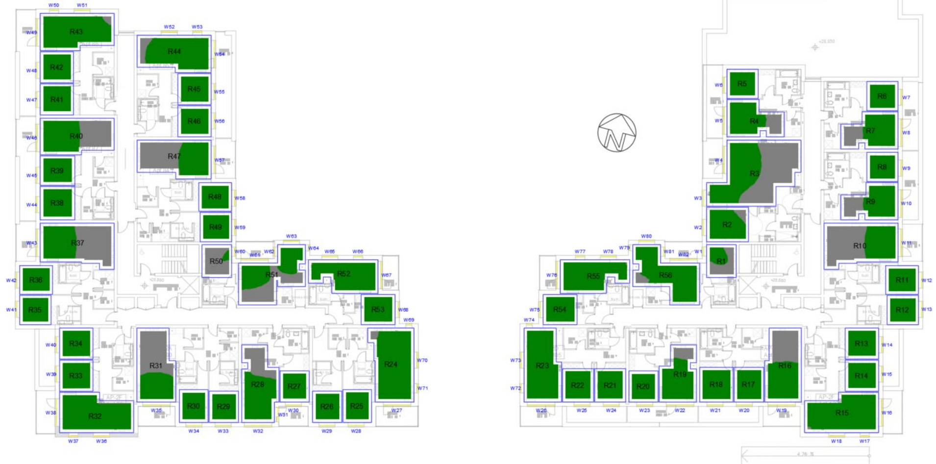
Figure 23: Resi. Apartment Third Floor sDA Contours
