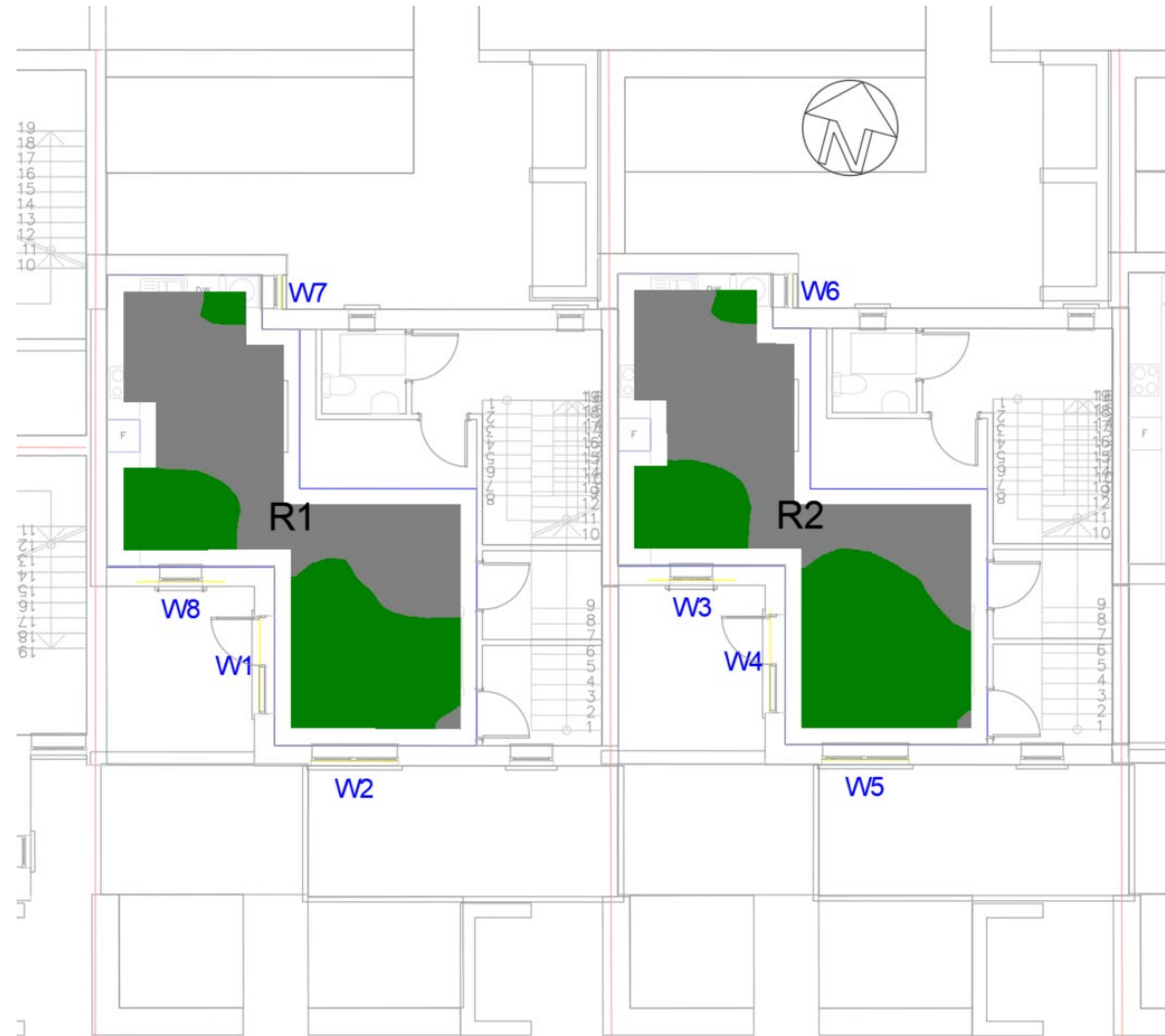
Figure 29: DP-03-04 First Floor sDA Contours
