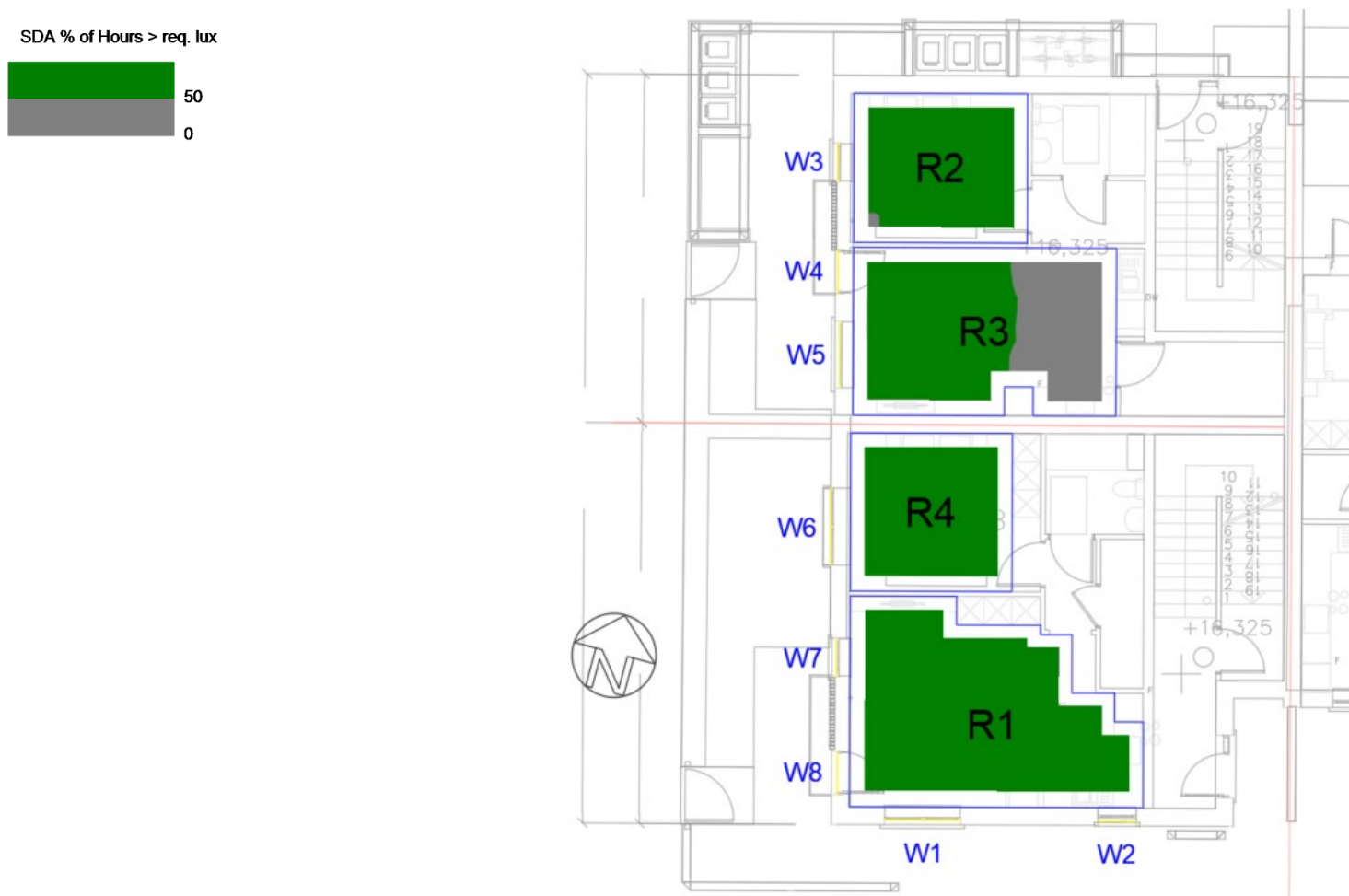
Figure 25: DP-01-02 Ground Floor sDA Contours
